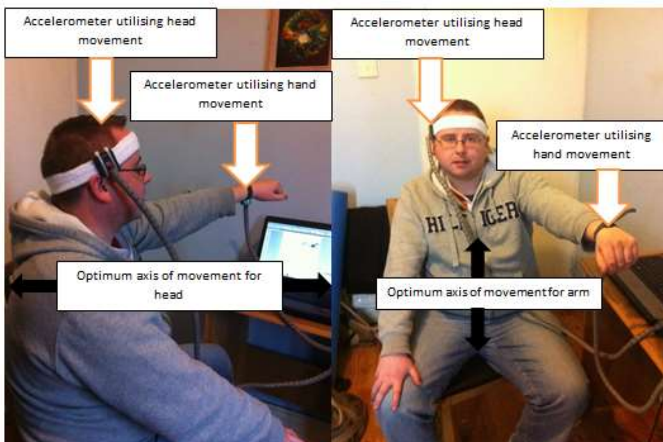
Figure 9 - Accelerometer Placement J.Fogarty 2014
