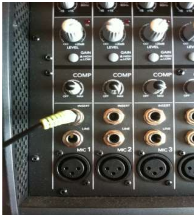
Figure B3 -Connecting Auxiliary Cable to PA System
